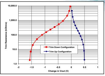
Figure E: Change in Output Voltage Graph.
