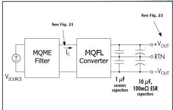
Figure 20: Test set-up diagram showing measurement points for Input Terminal Ripple Current (Fig 21) and Output Voltage Ripple (Fige 22).
