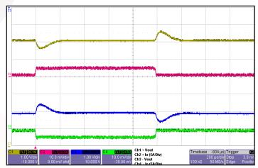
Figure 18: Output voltage response to step-change in total load current (10%-50%-10%) of total lout (max) split 50%/50%. Load cap: IµF ceramic cap and 10µF, 100 mW ESR tantalum cap. Ch 1: +Vout (1 V/div); Ch 2: +Iout (5A/div); Ch 4: -Vout (1 V/div); Ch 4: -Iout (5A/div).
