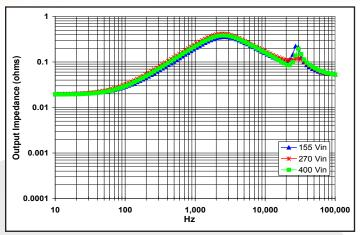
Figure 25: Magnitude of incremental output impedance (+Zout = +vout /+iout) for minimum, nominal, and maximum input voltage
