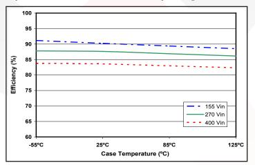
Figure 5: Efficiency at 60% load (3A load on +12V and 3A load on -12V) versus case temperature for V in =155V, 270V, and 400V.
