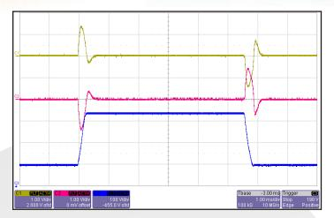
Figure 19: Output voltage response to step-change in input voltage (155V - 400V - 155V). Load cap: 10μF, 100 mW ESR tantalum cap and 1μF ceramic cap. Ch 1: +Vout (1V/div); Ch 2: -Vout (1V/div); Ch 3: Vin (100V/div).
