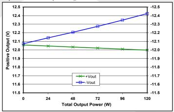
Figure 9: Load regulation vs. total output power from zero to to full load where +Iout equals three times -Iout at nominal input voltage and TCASE = 25°C.
