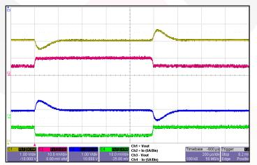
Figure 17: Output voltage response to step-change in total load current (50%-100%-50%) of total lout (max) split 50%/50%. Load cap: 1µF ceramic cap and 10µF, 100mW ESR tantalum cap. Ch 1: +Vout (1 V/div); Ch 2: +Iout (5A/div); Ch 3: -Vout (1 V/div); Ch 4: -Iout (5A/div).
