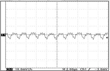
Figure 21: Input terminal current ripple, ic, at full rated output current and nominal input voltage with SynQor MQ filter module (100 mA/div). Bandwidth: 20MHz. See Fig 20.
