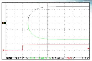
Figure 14: Turn-on transient at zero load current (5 ms/div). Input voltage pre-applied. Ch 1: +Vout (5V/div); Ch 2: -Vout (5V/div); Ch 3:
