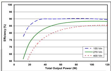
Figure 1: Efficiency vs. output power, from zero load to full load with equal load on the +12V output and 50% load on the -12V output at minimum, nominal, and maximum input voltage at  $25^{\circ}$ C.
